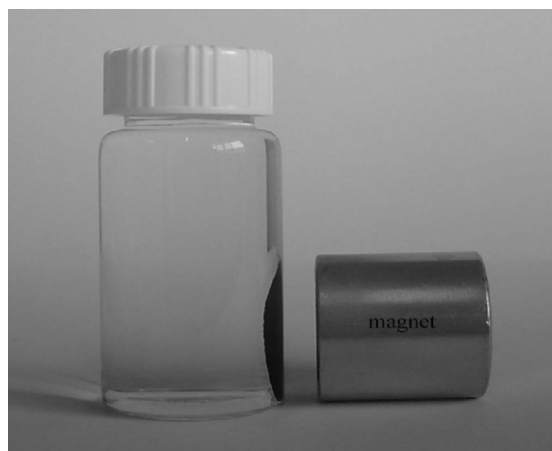
Fig. 1. Photograph of MWCNTs/iron oxides/CD magnetic separation.
